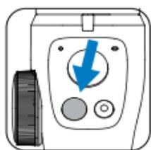
3. To turn on, press and hold the power button for three seconds.
