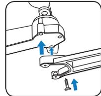
2. To remove the rotor guard, please press the middle part of rotor guard first, then take the rotor guard out.
