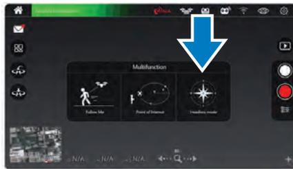
3. When headless mode is enabled, the drone will move in the direction of the remote control, regardless of its orientation. This makes it easy to bring the drone home when it is far away from you.
